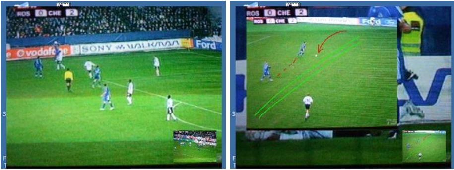
Fig. 4. Left: A thumbnail of the annotated frame is presented to indicate that an ink note is available. Right: The ink note is presented when the user selects the proper button on the digital TV remote control.
